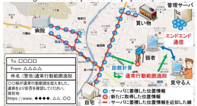
Fig.2. Abnormality detection method.
