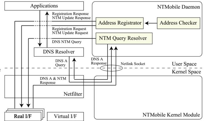
Fig. 6. System model of NTM mobile node.
