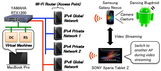
**Figure 3: Configuration of demonstration.**
