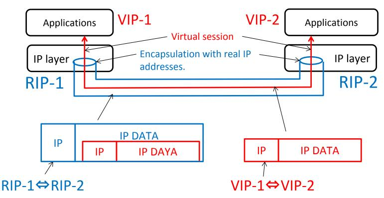
Real IP addresses change if NAT exists on the communication route. Real IP addresses change if the access network changes. Virtual IP addresses never change.
